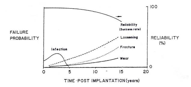
Failure modes also depend on the type of implant and its location and function in the body
